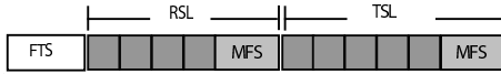
Figure 2: A node's transmission schedule structure. The slots are not contiguous in time.
